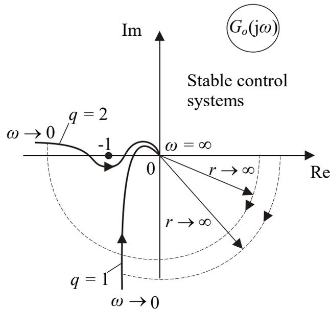
Fig. 3.13 – Nyquist plots  $G_o(j\omega)$  for stable control systems with  $q = 1$  and  $q = 2$
