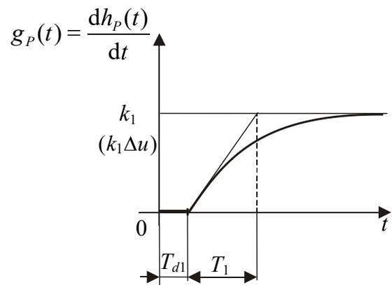
Fig. 3.7 – Identification of integrating plants on the basis of:
