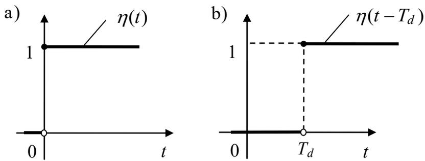
Fig. 2.7 – Unit step: a) undelayed, b) delayed
