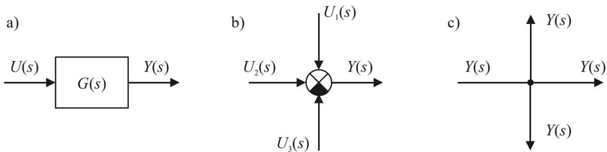
Fig. 2.13 – Representation: a) a linear dynamic system by a block, b) variable addition or subtraction by a summing node, c) variable branching by an information node
