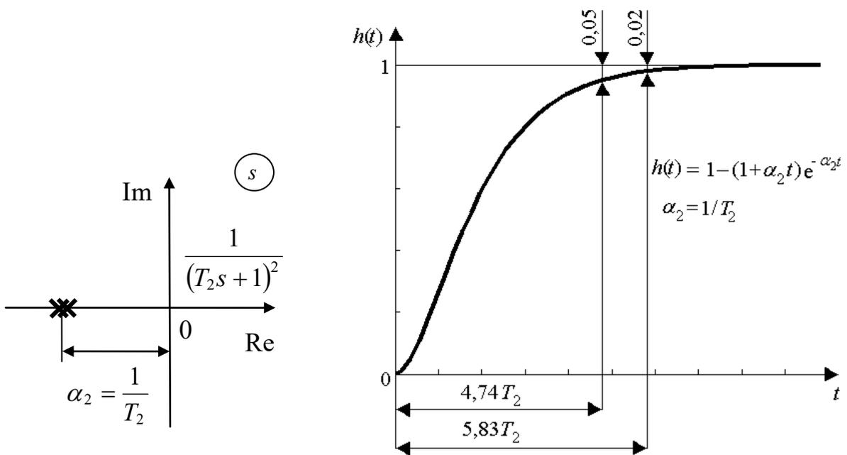
Fig. 4.13 – Influence of stability degree (damping) on the step response and settling time for a non-oscillating system of: a) the first order, b) the second order
