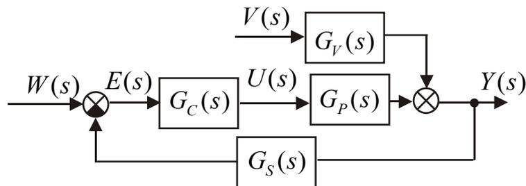
Fig. 3.1 – Block diagram of a common control system
