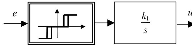
Fig. 6.5 – Three-position controller with integrating device
