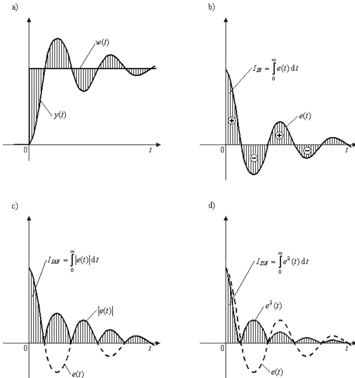
Fig. 4.6 – Geometrical interpretation of integral criteria: a) control area, b) integral of error  $I_{IE}$ , c) integral of absolute error  $I_{IAE}$ , d) integral of squared error  $I_{ISE}$
