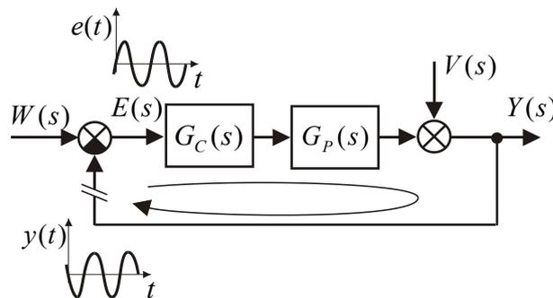
Fig. 3.11 – Control system on stability boundary
