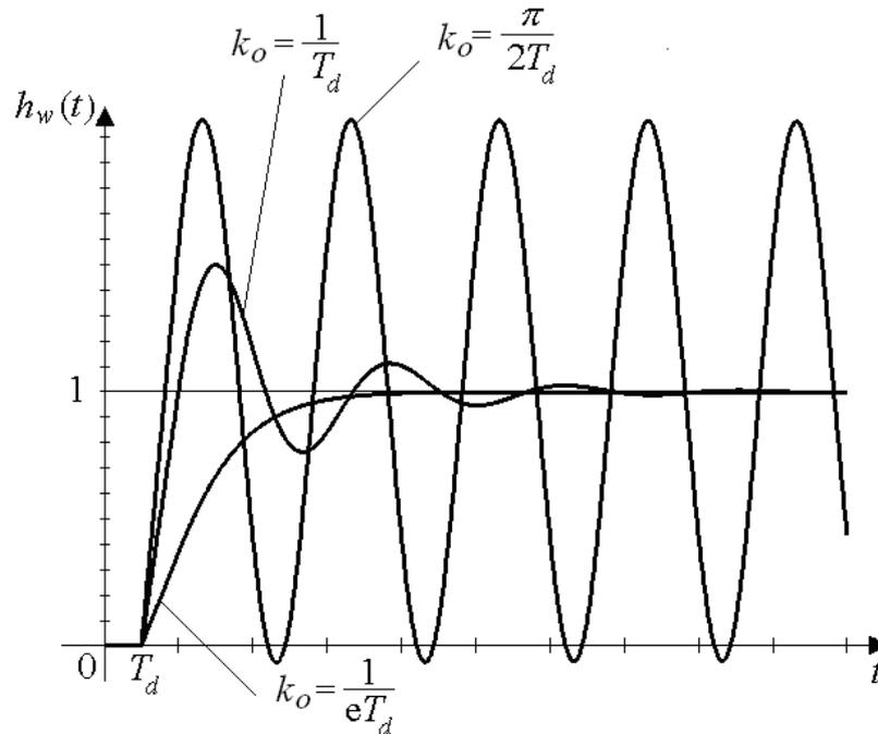
Fig. 4.20 – Influence of open-loop gain  $k_o$  on control system step responses
