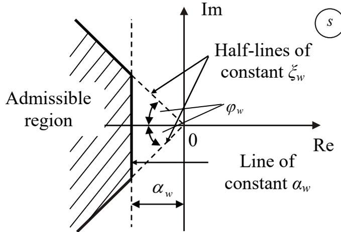
Fig. 4.14 – Determination of admissible region for control system poles
