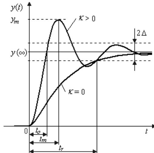
Fig. 4.5 – Servo (setpoint) responses with marked control performance indices
