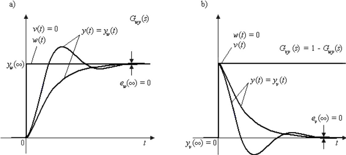
Fig. 4.1 – Control system step responses in the case of zero steady-state errors: a) servo (setpoint) responses, b) regulatory responses for disturbance variable in the plant output
