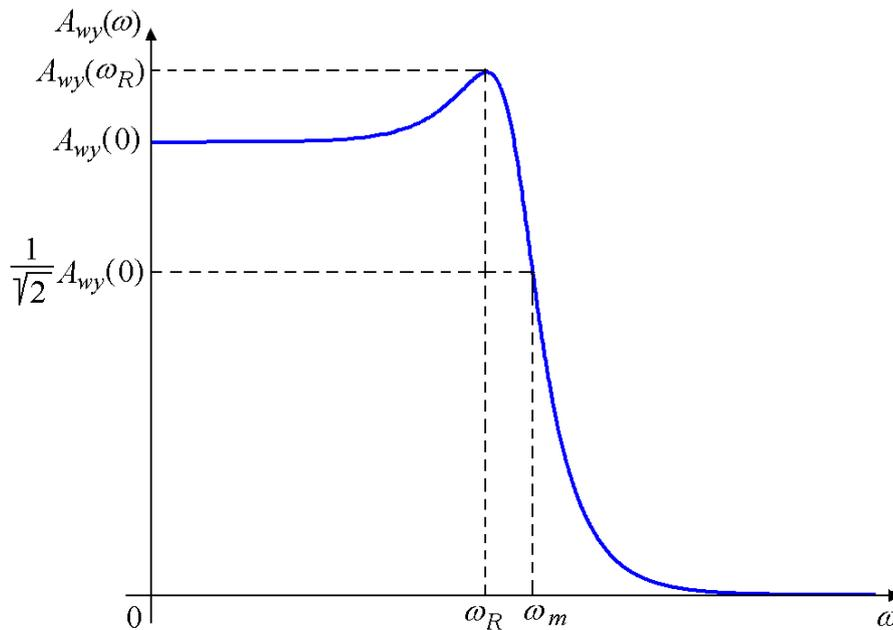
Fig. 4.8 – Magnitude response of a control system
