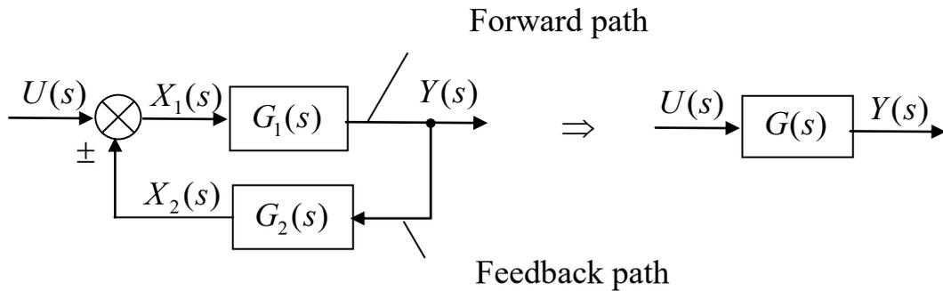
Fig. 2.16 – Feedback interconnection of blocks
