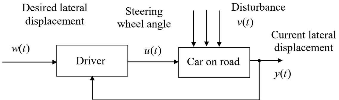
Fig. 1.1 – Control of car on a road
