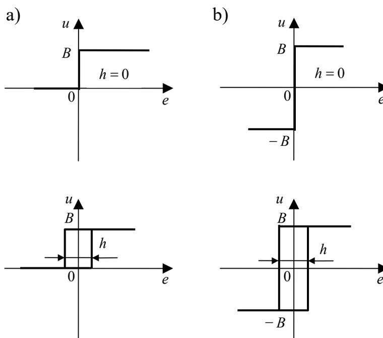
Fig. 6.1 – Different characteristics of a two-position controller: a) asymmetric without hysteresis ( $h = 0$ ) and with hysteresis ( $h > 0$ ), b) symmetric without hysteresis ( $h = 0$ ) and with hysteresis ( $h > 0$ )
