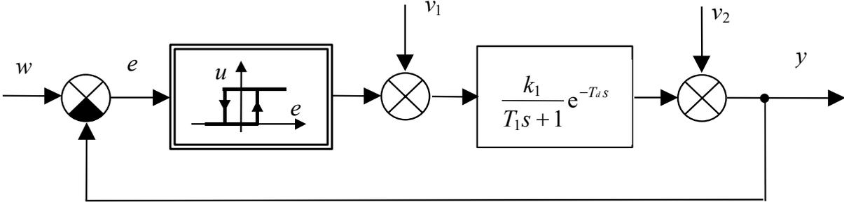
Fig. 6.3 – Control system with ON-OFF controller
