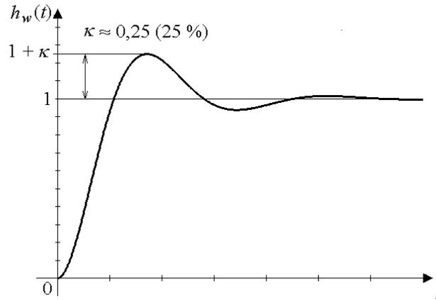
Fig. 4.16 – „Average“ step response of control system tuned by experimental Ziegler – Nichols methods
