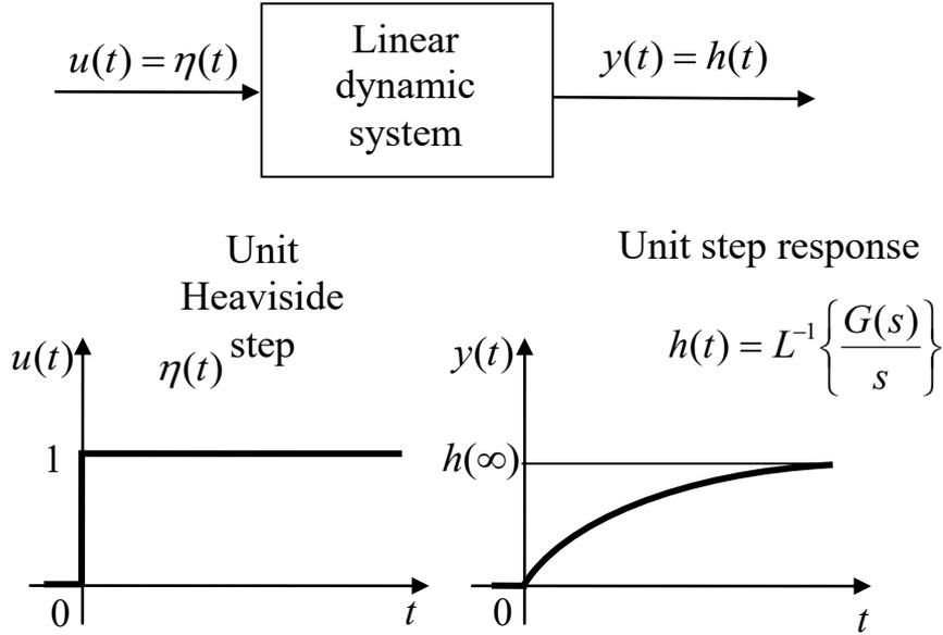
Fig. 2.9 – Unit step response of a linear dynamic system
