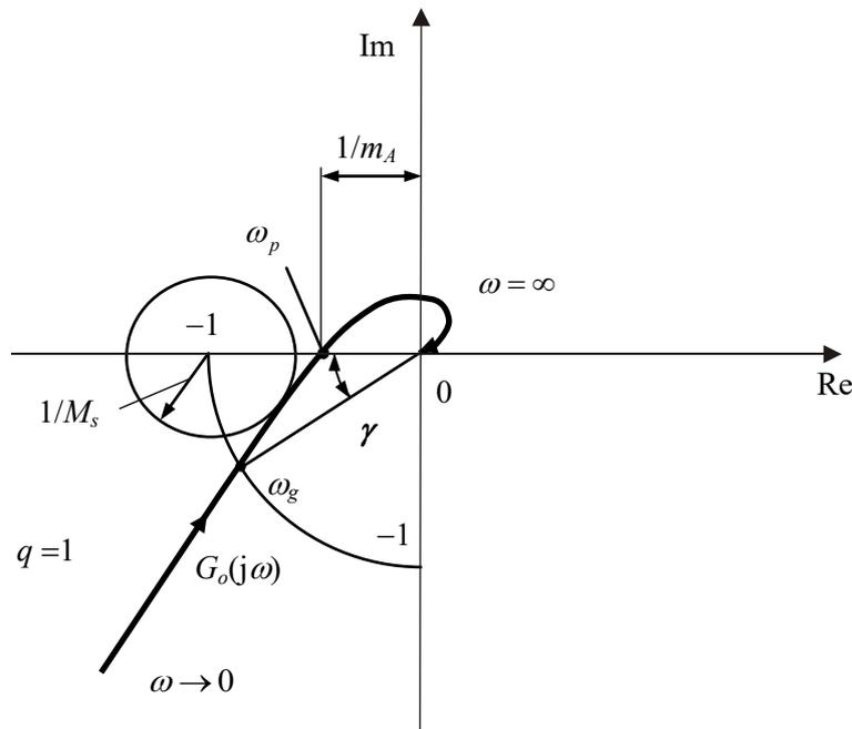
Fig. 4.10 – Geometrical interpretation of the maximum of the sensitivity function modulus
