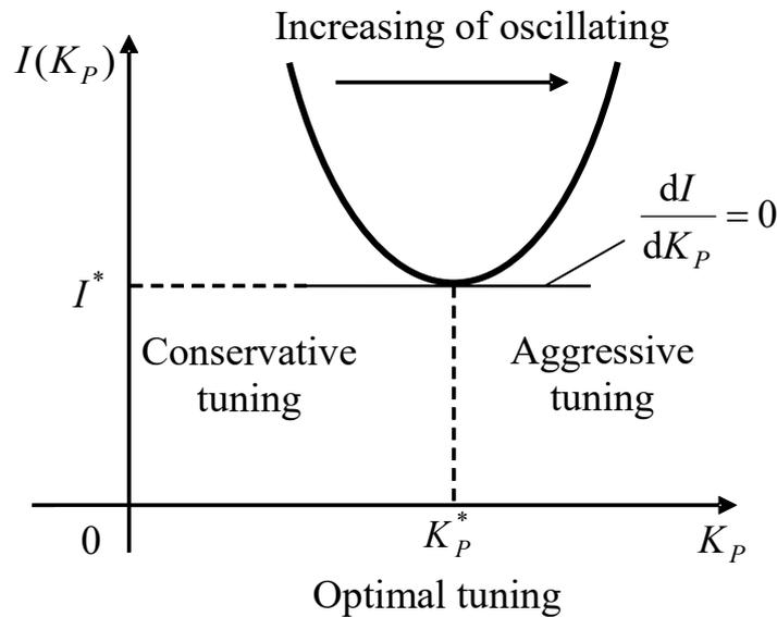
Fig. 4.15 – Dependence of performance index  $I$  on controller gain  $K_P$
