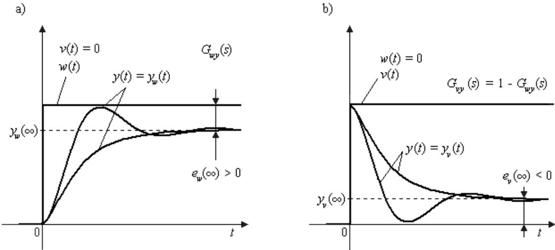
Fig. 4.2 – Control system step responses in case non-zero steady-state errors: a) servo (setpoint) responses, b) regulatory responses for disturbance variable in plant output
