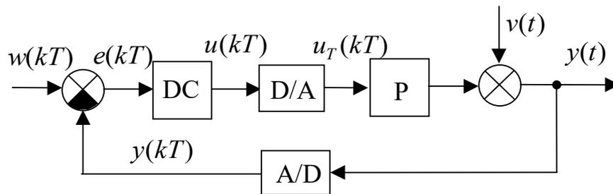
Fig. 5.2 – Control system with a digital controller
