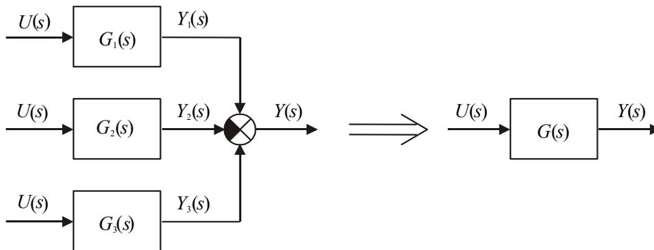
Fig. 2.15 – Parallel interconnection of blocks
