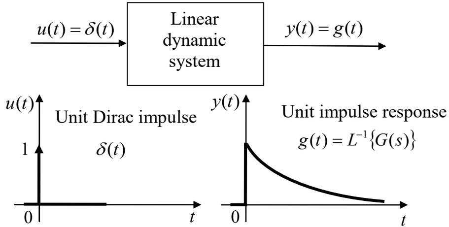
Fig. 2.8 – Unit impulse response of a linear dynamic system
