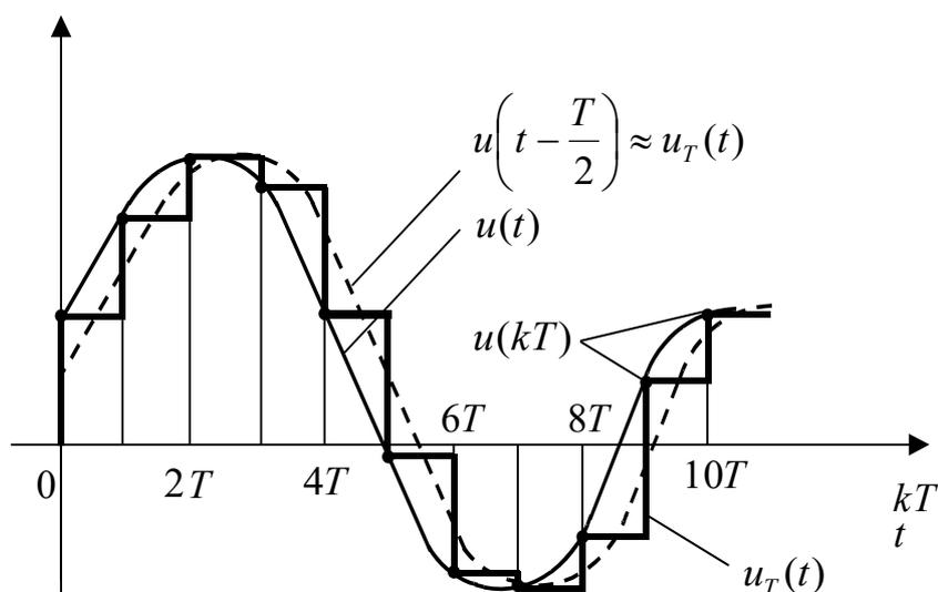
Fig. 5.3 – Control variable courses in a control system with a digital controller
