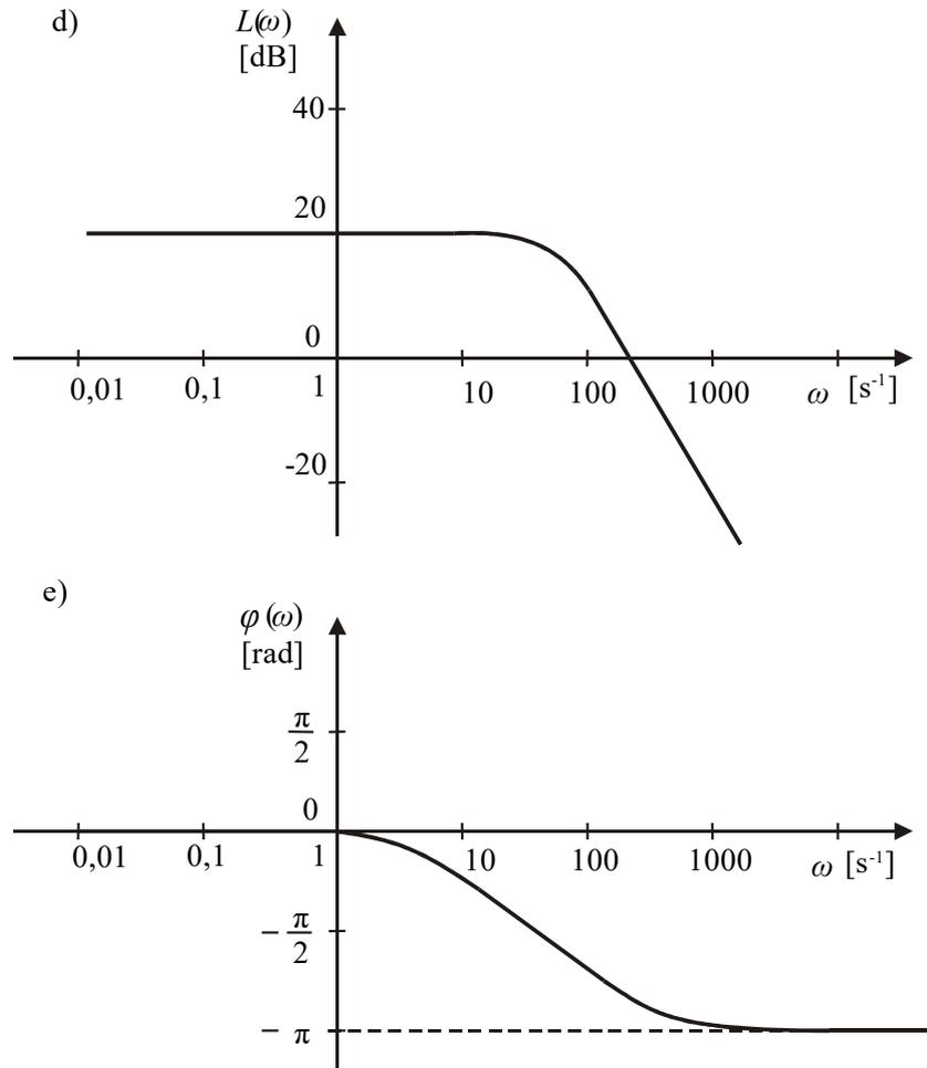
Fig. 2.11 – Frequency responses: d) Bode magnitude plot, e) Bode phase plot
