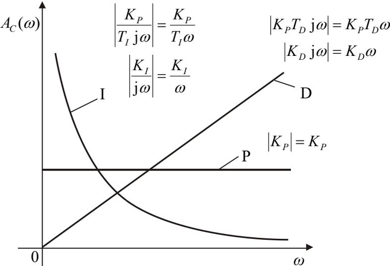
Fig. 3.3 – Dependence of partial controller components P, I and D of PID on angular frequency
