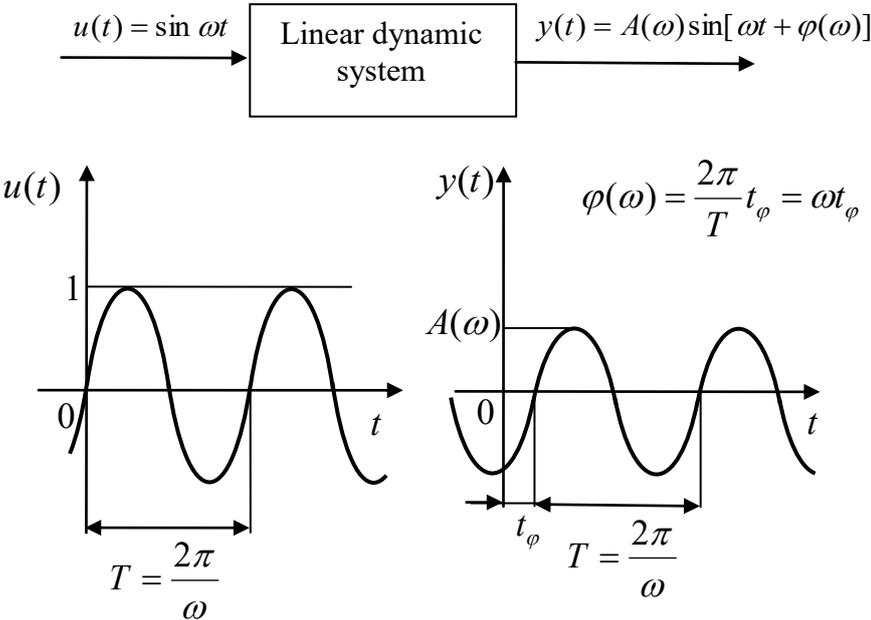
Fig. 2.12 – Interpretation of a frequency response of a linear dynamic system
