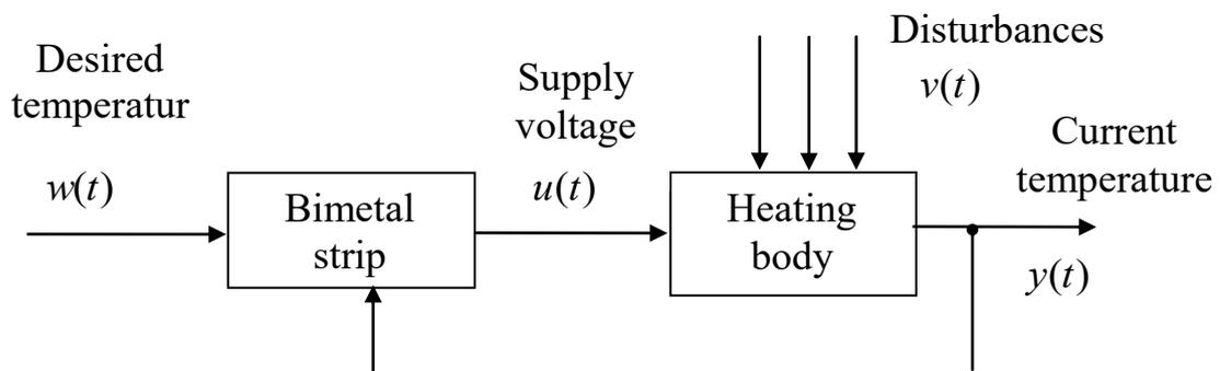
Fig. 1.3 – Iron temperature control
