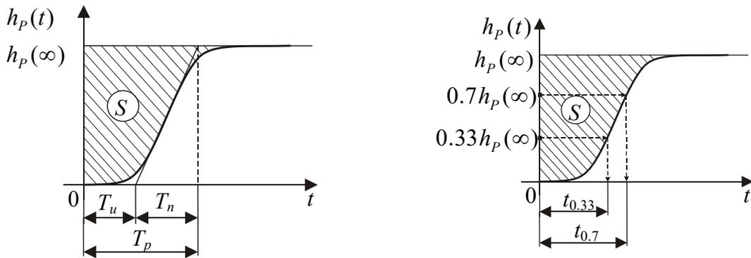
Fig. 3.6 – FOPTD plant identification on the basis of:
