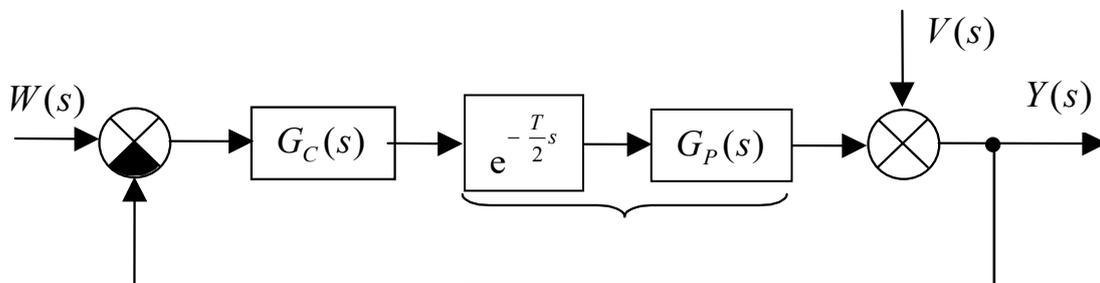
Fig. 5.4 – Substitute control system with the digital controller
