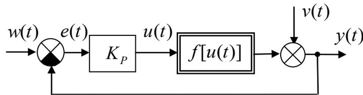
Fig. 1.9 – A closed-loop control system with a non-linear plant
