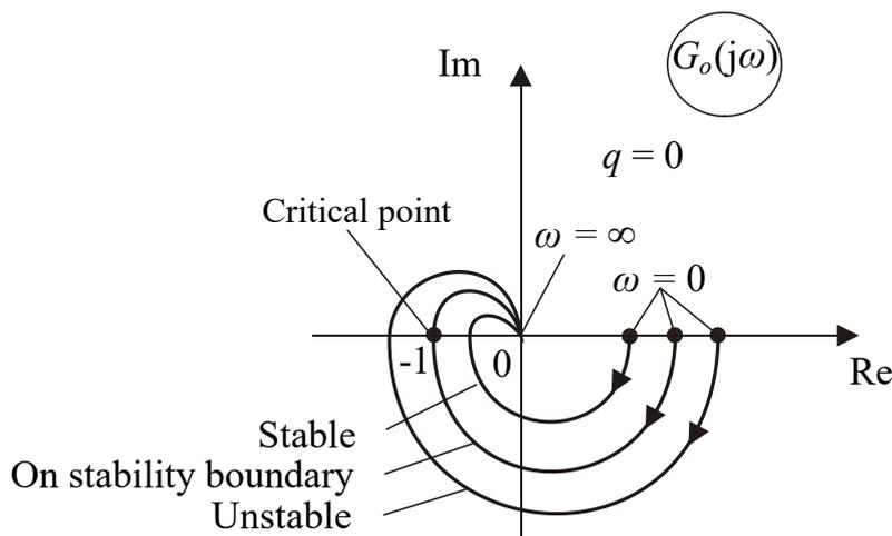
Fig. 3.12 – Nyquist plots  $G_o(j\omega)$  for control system with  $q = 0$
