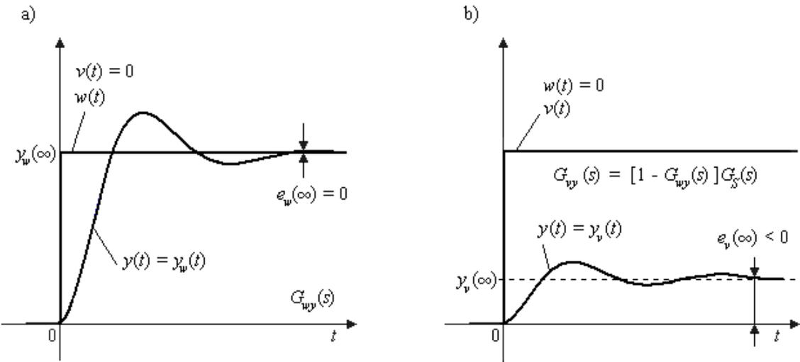
Fig. 4.4 – Control system step responses for a controller without an integral component and integrating plant: a) servo (setpoint) response, b) regulatory response for a disturbance variable in the plant input
