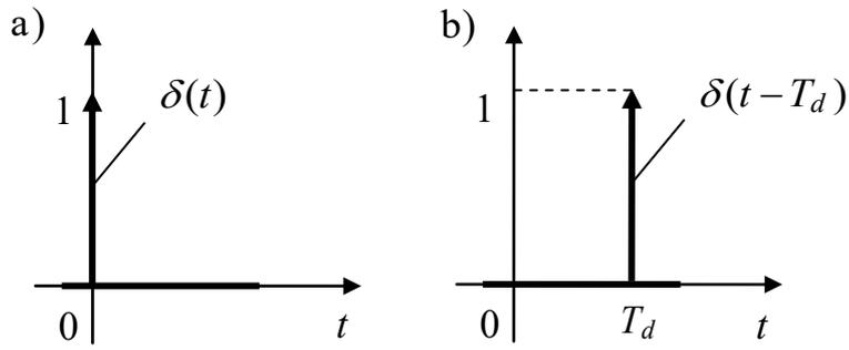
Fig. 2.6 – Unit impulse: a) undelayed, b) delayed
