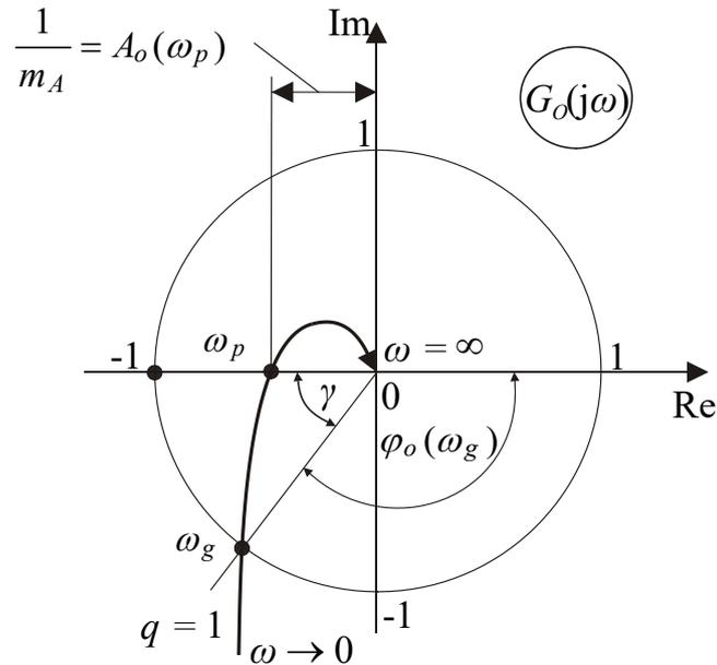
Fig. 3.14 – Gain margin  $m_A$  and phase margin  $\gamma$
