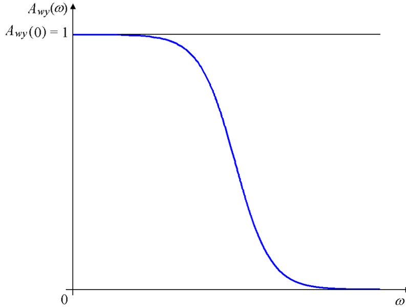
Fig. 4.19 – Desired course of the modulus of a frequency control system transfer function
