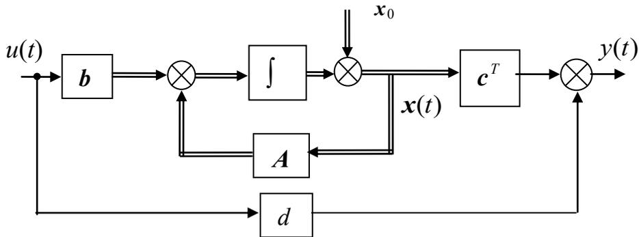
Fig. 2.10 – Block diagram of a SISO state space model
