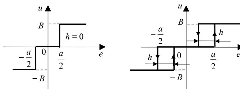
Fig. 6.2 – Characteristic of a symmetric three-position controller without hysteresis ( $h = 0$ ) and with hysteresis ( $h > 0$ )
