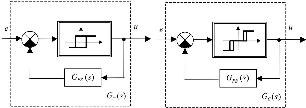
Fig. 6.6 – Two- and three-position controller with dynamic feedback
