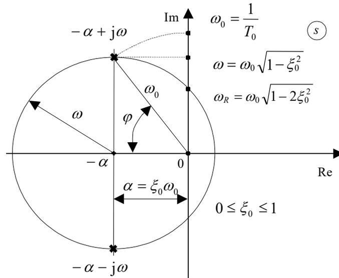
Fig. 4.11 – Geometrical interpretation of the second order oscillating system parameters
