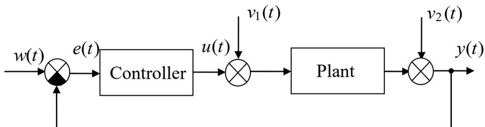
Fig. 1.5 – Closed-loop control system
