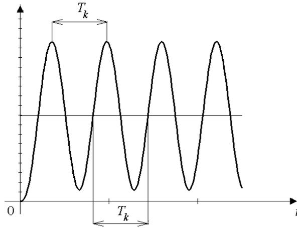
Fig. 4.17 – Determination of ultimate period  $T_c$
