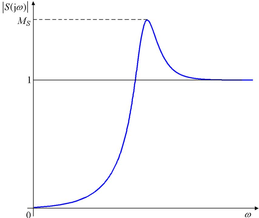
Fig. 4.9 – Course of the modulus of the sensitivity function
