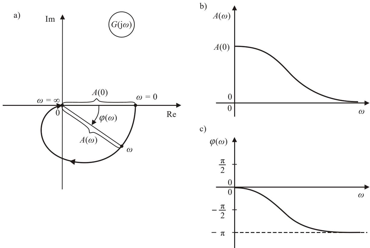
Fig. 2.11 – Frequency responses: a) polar plot, b) magnitude frequency response, c) phase frequency response
