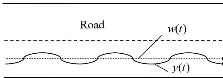
Fig. 1.2 – Courses of a current  $y(t)$  and desired  $w(t)$  car displacement from the middle of the right side of the road
