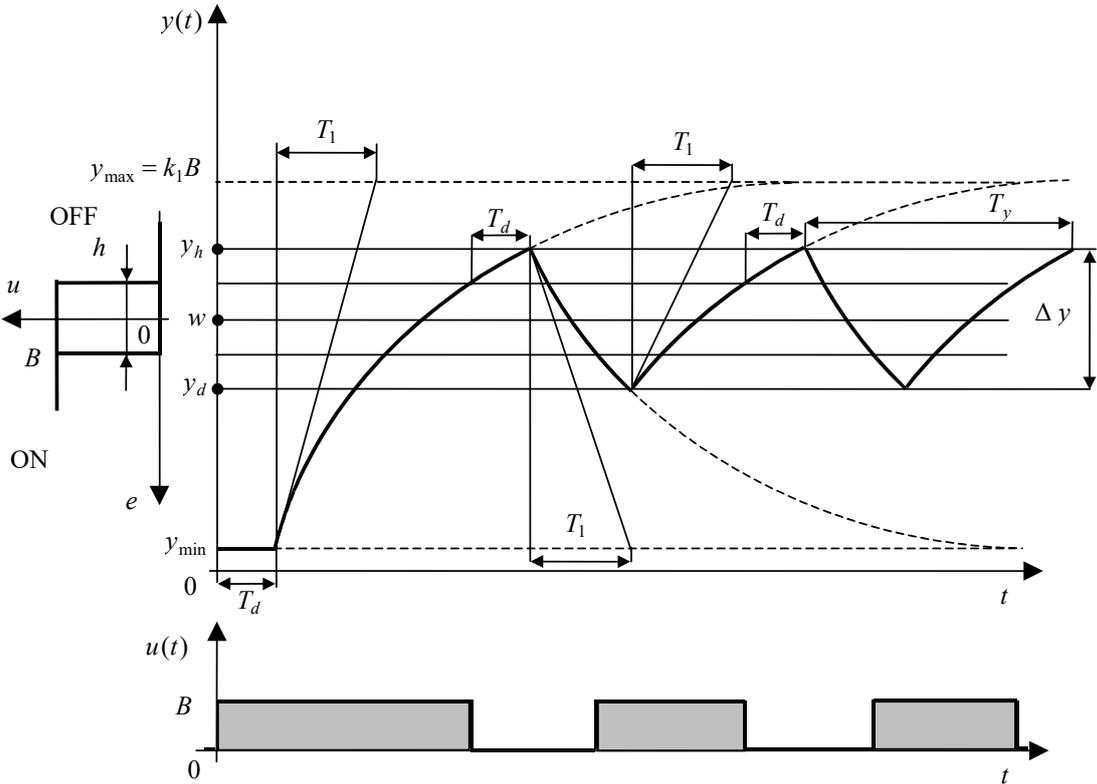
Fig. 6.4 – Courses of controlled  $y(t)$  and control  $u(t)$  variables in control system with an ON-OFF controller
