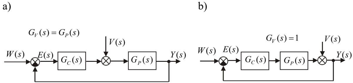
Fig. 3.2 – Control system with disturbance: a) in the input of a plant, b) in the output of a plant
