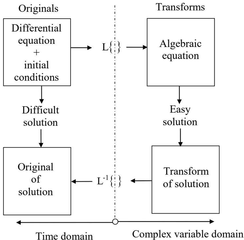
Fig. 2.4 – Solving a differential equation by the Laplace transform
