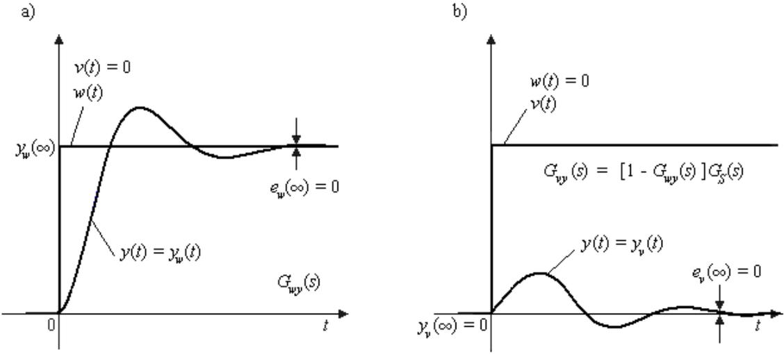
Fig. 4.3 – Control system step responses for a controller with integral component and proportional plant: a) servo (setpoint) response, b) regulatory response for a disturbance variable in plant input
