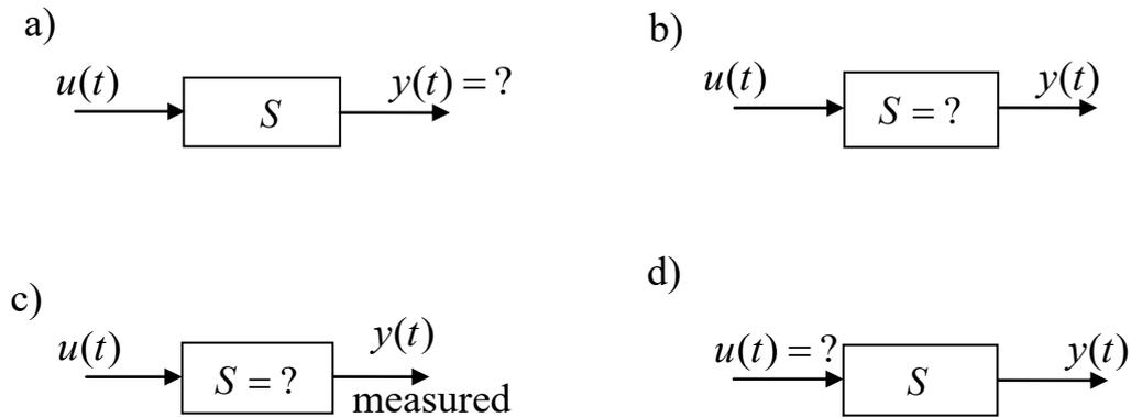
Fig. 1.11 – Basic problems in automatic control: a) analysis, b) synthesis, c) identification, d) control
