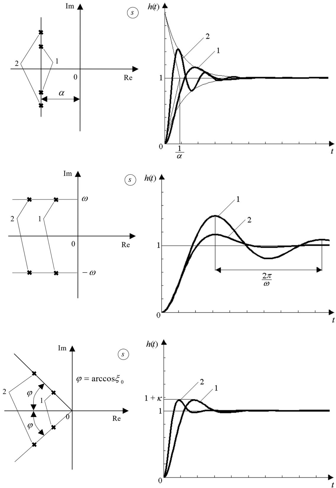
Fig. 4.12 – Influence of complex conjugate poles of the second order oscillating system on its step responses
