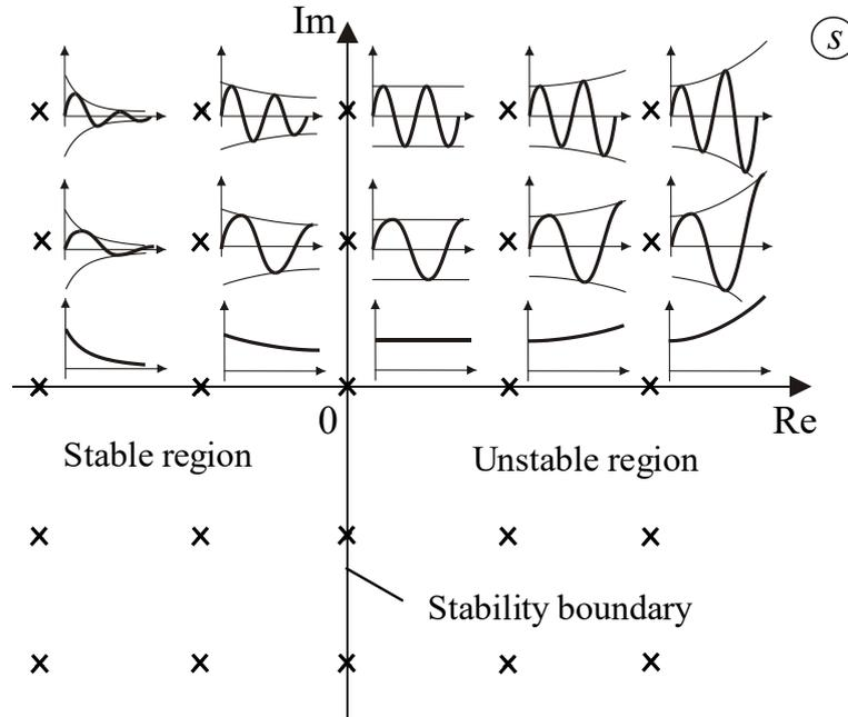
Fig. 3.8 – The influence of the position of control system poles on the transient part of the response
