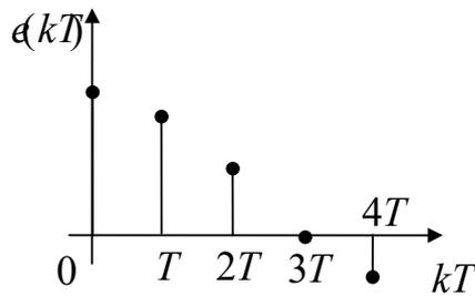
Fig. 5.1 – Control error course in a control system with a digital controller
