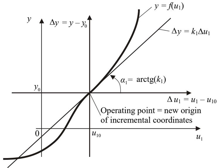
Fig. 2.17 – Geometrical interpretation of linearization by a tangent line for one input
