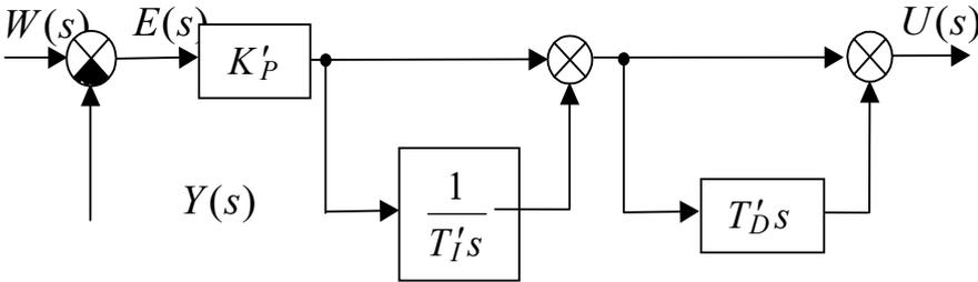
Fig. 3.4 – Block diagram of a PID controller with a structure: a) parallel (without interaction), b) serial (with interaction)
