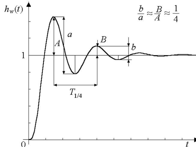
Fig. 4.18 – Control system tuning by the quarter-decay method
