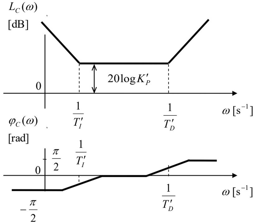
Fig. 3.5 – Bode plots of  $PID_i$  controller
